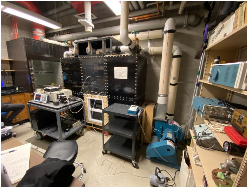
Figure 1: Marple-type dust chamber setup.
