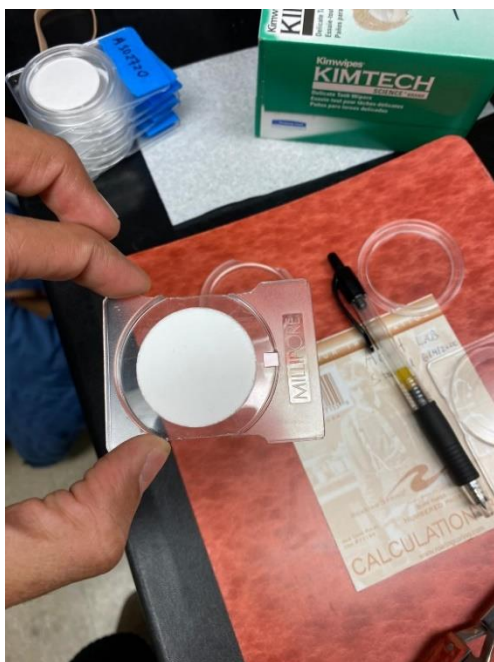
Figure 8 Filter holder used in the FTIR instrument.
