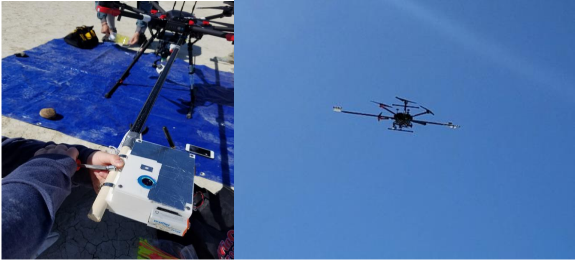
Figure 9: Configuration of instrument mounted to UAS. A long pole, approximately 2 m in length, was used to extend the instrument away from the body of the aircraft. This was done to limit the effects of the aircraft on albedo measurements, specifically those which would change the surrounding radiation field.
