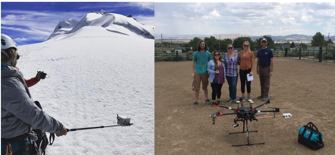
Figure 8: Left photo. Undergraduate Chris Stevens using the Albedometer prototype mounted to the end of a trekking pole in handheld mode on a glacier in the Cordillera Blanca, Peru. Right photo. Albedometer mounted to end of copper pole on DJI Matrix 600 Pro hexacopter at Silver Knoll Ranch for a test flight.
