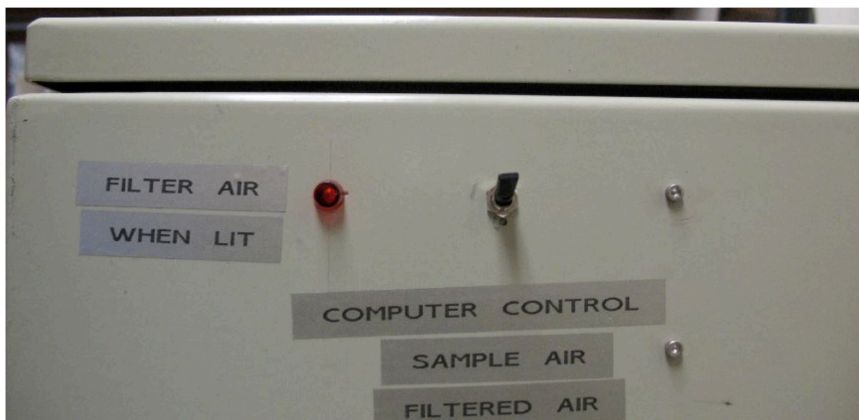
Figure 4. Instrument front panel. The switch has 3 positions. When up, the computer controls the inlet switch choice between sample air and filtered air. When in the middle position the inlet is set for sample air. When down, the inlet is set for filtered air. The inlet switching device in the instruments gets hot when left on the 'filtered air' setting for longer than 10 minutes, and the instrument will shut down when a thermal switch activates. It is generally best NOT to use the filtered air setting, except for brief periods of a few minutes.
