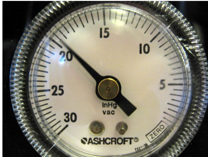
Figure 2. Pressure gauge indicating vacuum level. For proper operation the pressure should be between 15 and 30. If it is below 15, check to make sure the pump line is not leaking.
