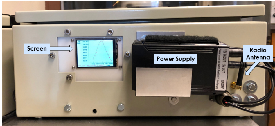
Figure 13. Photograph of the side of the prototype instrument enclosure. A screen is mounted to allow for monitoring of instrument operations. The power supply is mounted on the outside for easy replacement. The radio antenna transmits collected data serially.
