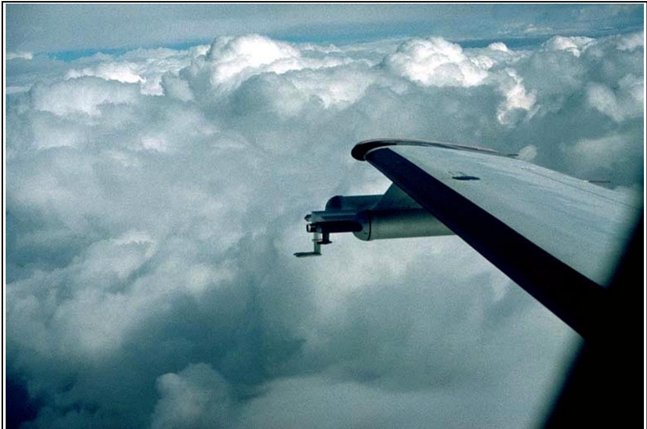
Figure 2. Cloudscope mounted on the outer pod of the UND Citation.
