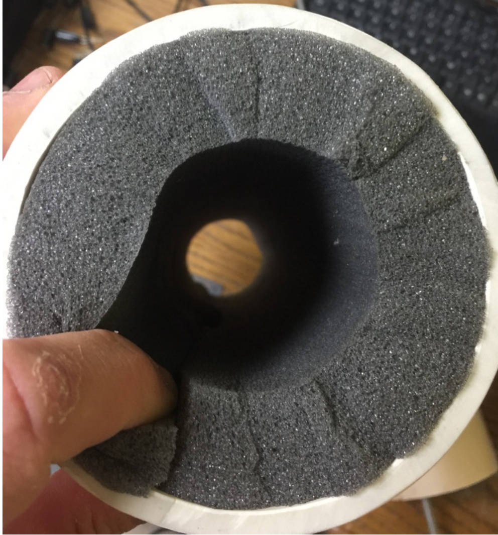
Figure 8. Photo of a thick foam layer at the PVC wall. The screen was left out for this photo.
