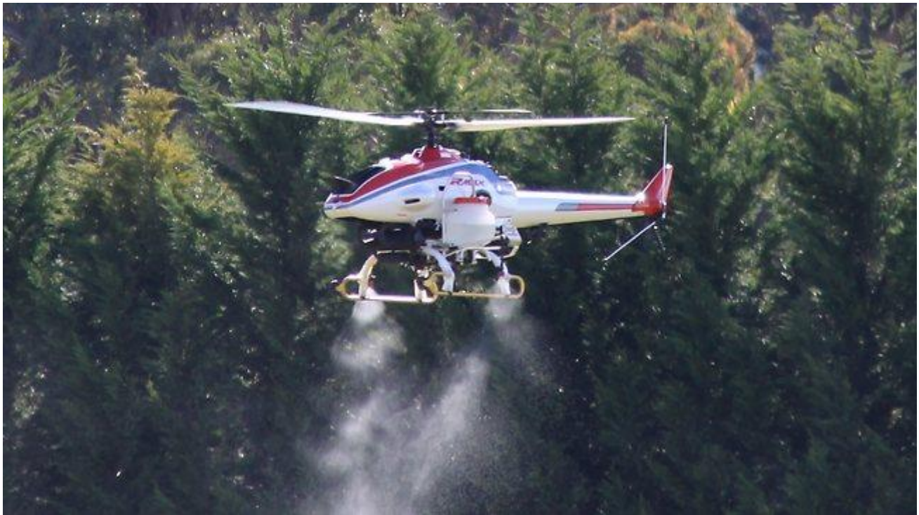
Figure 6. The Yamaha RMAX VTOL aircraft, shown with a pesticide/herbicide application sprayer payload used in precision agriculture. Image courtesy of Yamaha Motor Australia.
