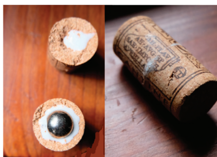
Figure 4. The picture on the left shows the two halves of the cork, with the hemispherical dimples carved into them, both filled with vinyl glue and one of them hosting the metal sphere. The picture on the right shows the assembled cork. In this configuration, the cork density was still smaller than that of water and it was necessary to cut thin slices of the cork to make it slightly denser than water.
