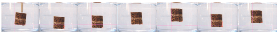
Figure 2. Shots of the cork during oscillation induced by a slight initial push. A video is included as supplemental material (video 1) ( https://stacks.iop.org/EJP/42/055011/mmedia ).
