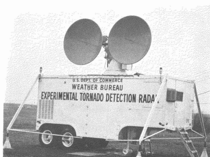
FIGURE 1.—The 3-cm. continuous-wave Doppler radar equipment trailer.
