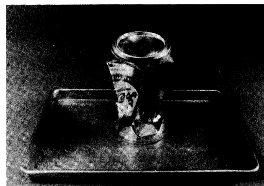
Figure 6.1 When a can filled with hot water vapor is placed in a shallow pan filled with cooler water, the can is crushed because of the pressure difference between its inside and its outside. That outside is atmospheric pressure. That inside is initially atmospheric pressure but drops as the water vapor condenses onto the cooled walls of the can.
