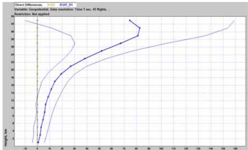
Figure 4.4. Comparison of GPS-based geopotential height with the RS41 and sensor-based geopotential height with the RS92 radiosonde, using the RS92 as the reference. Showing average differences and standard deviation of differences (thin lines) from 45 flights.
