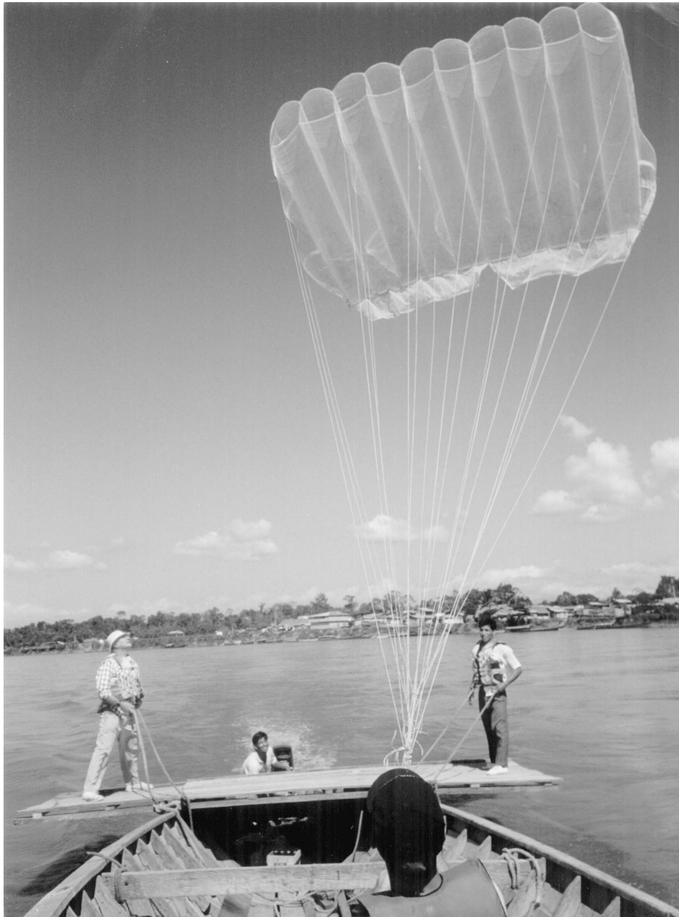
Figure 5. Kite launch from a small outboard boat on the Marañon River in Peru's Upper Amazon Basin. In this case, the relative wind velocity is controlled by the boat's speed and the river current.
