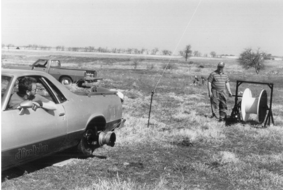
Figure 3. Photograph showing one possible winching technique. In this case, the kite tether is brought down through a pulley to a capstan mounted on the rear axle of a vehicle. The line is then wound onto a take-up reel under light tension. The power necessary to reel in the kite is provided by the vehicle.
