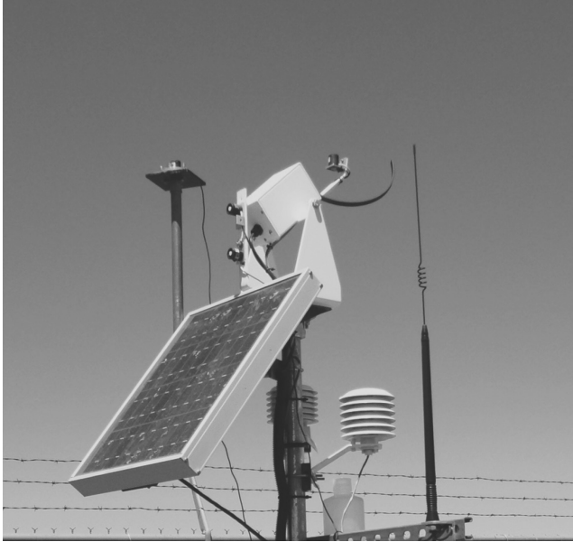
FIGURE 7.3 The Irradiance, Inc. rotating shadowband radiometer version 2 (RSR2). (Courtesy of Ed Kern.)
