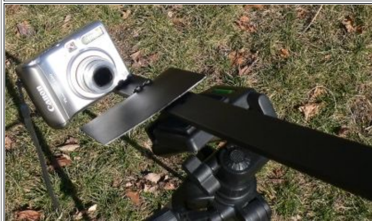
Figure 1. Tripod fixture for photographing the solar aureole.
