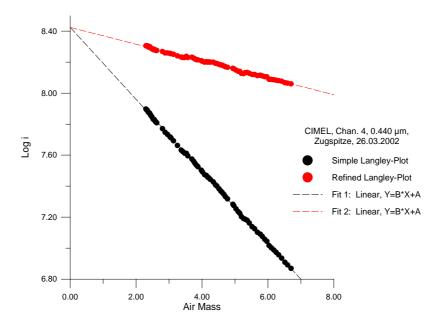
The refined Langley-plot is the same, corrected for the Rayleigh scattering, e.g. divided by the transmission for the Rayleigh scattering.
