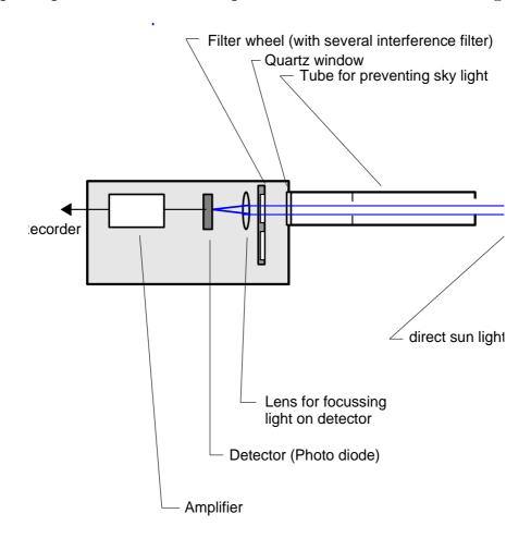
A diaphragma tube determines the viewing angle of the instrument, which is slightly larger than the angle of the sun disk (0.5 deg). Most instruments use 1.0 deg.
