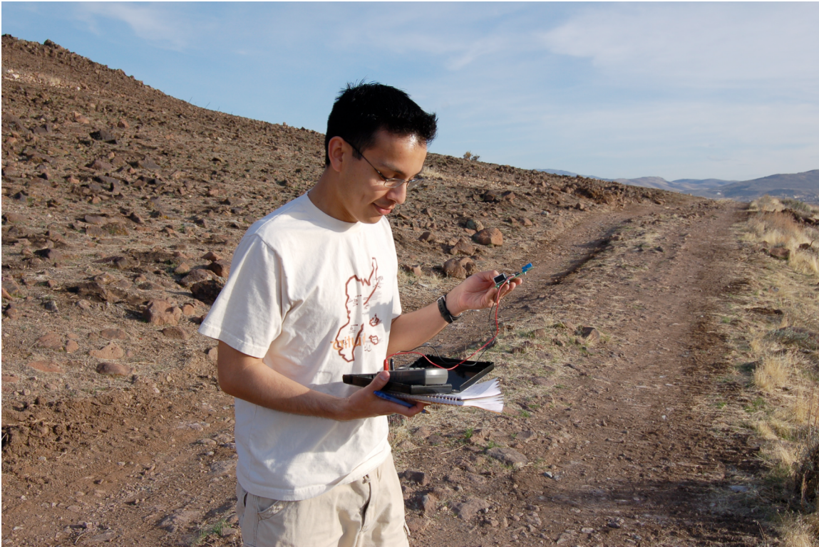
Figure 4: Photo of Mark Rincon using the sun photometer to take measurements.
