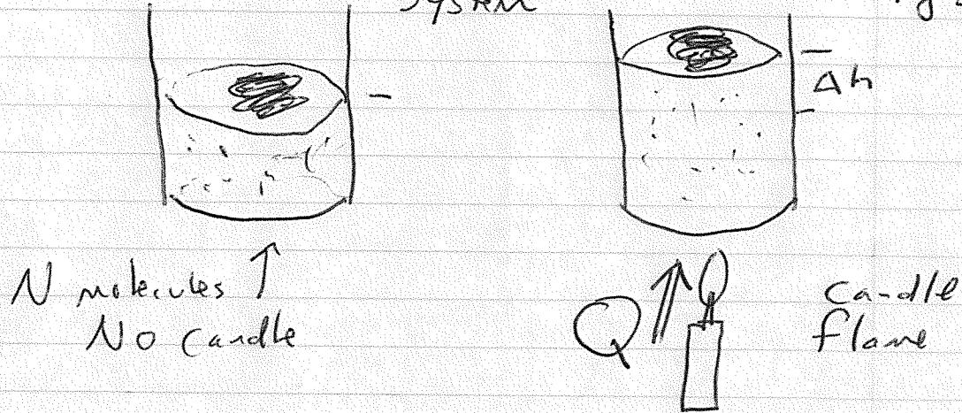
The candle both causes the molecules to move around faster, and the cap to move up. The increase in potential energy of the cap is
